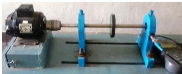
Fig. 1. FFT analyzer connected with rotor setup.
