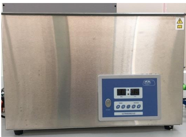
Fig. 2. The 3000868 - Ultrasons-HD (JP SELECTA in SPAIN) used for formulating Al 2 O 3 nanofluids.
