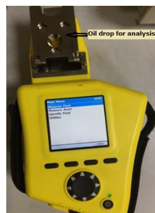
Fig. 2. Oil scanning using Fluid Scan Q1000 device.
