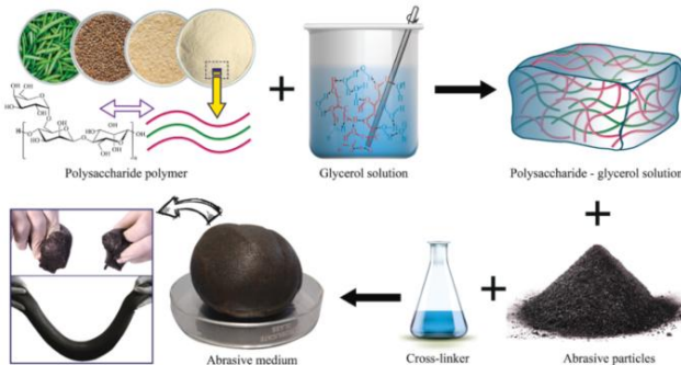
Fig. 2. Schematic illustration of the abrasive medium preparation.
