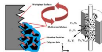
Fig. 4 Diagram of the velocity and force components in traditional AFM
