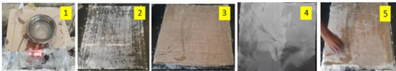
Fig. 2. Steps involved in the hand layup technique.
