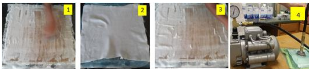
Fig. 3. Steps involved in the vacuum bag technique.
