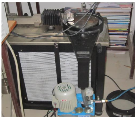
Fig. 5. Pin on Disc Machine with Specimen.
