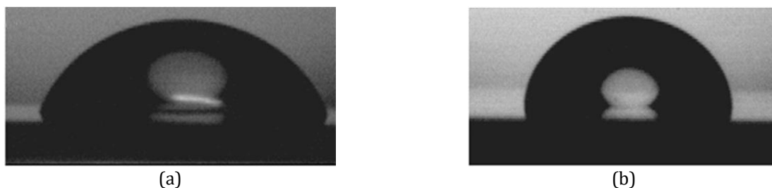
Fig. 4. Water droplets on (a) NDLC and (b) PtRuNDLC-NC coating surfaces.
