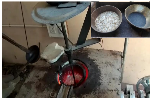
Fig. 1. Stir Casting Process with Reinforcement particles.
