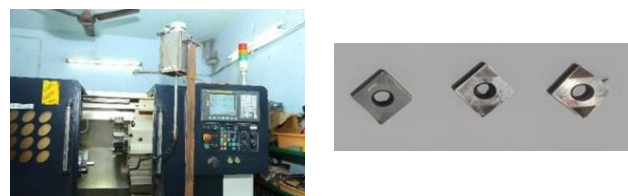
Fig. 4. CNC Machine with solid lubrication Device and Cutting inserts with micro-hole.
