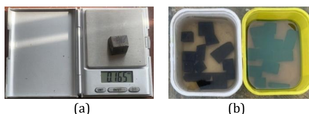
Fig. 5 (a) Camry pocket size weighing meter, (b) Absorption test.
