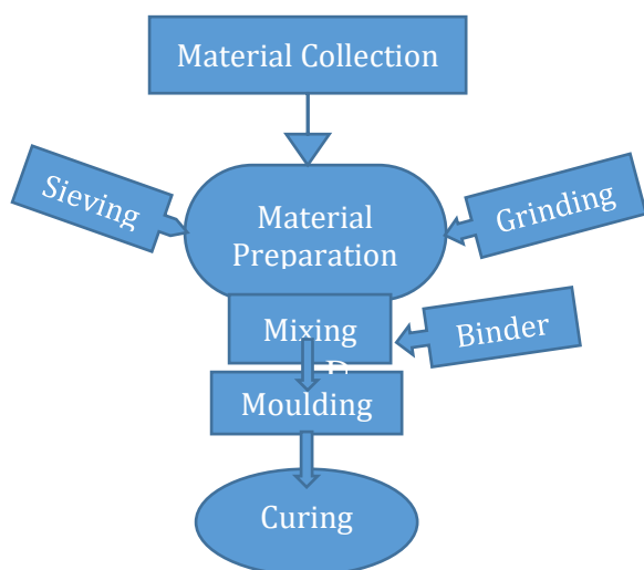
Fig. 2. Brake pad production flowchart.
