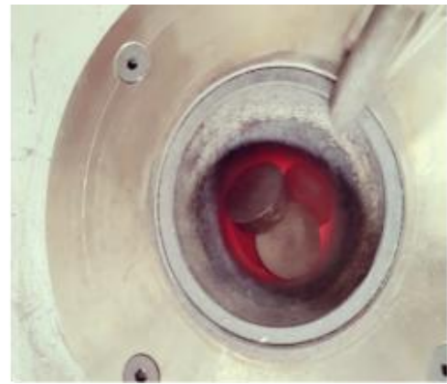
(b) Furnace used for fabrication of Al-Graphite MMC
