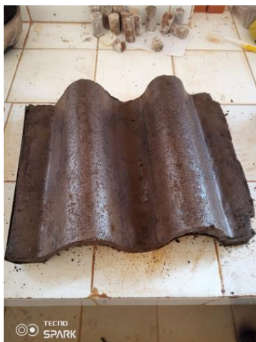
Fig. 11. Processed river sand-chamotte-PET plastic-based composite roofing tile prototype with 30 % of PET plastic+10 % of chamotte+ 60 % of sand.
