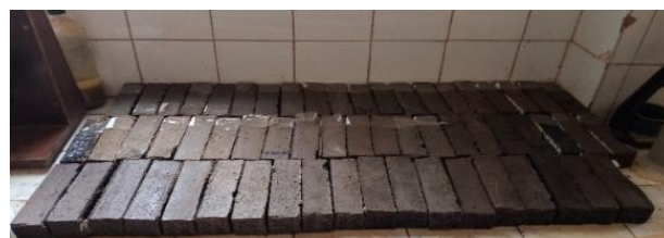
Fig. 4. Formulated river sand-chamotte-plastic composite roofing tile's test specimens (4 cm x 4 cm x16 cm) size.
