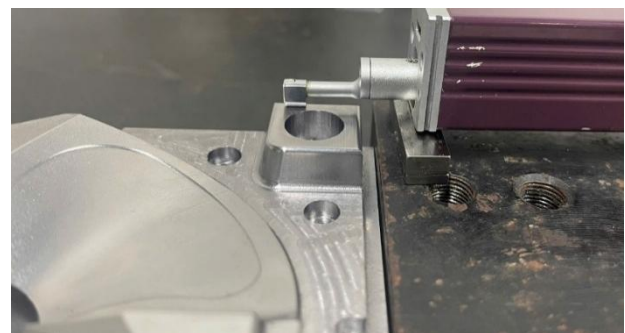
Fig. 2. Contact measurement method using a planar-touch stylus probe
