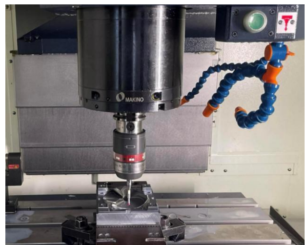
Fig. 6. Probing process on a CNC machine
