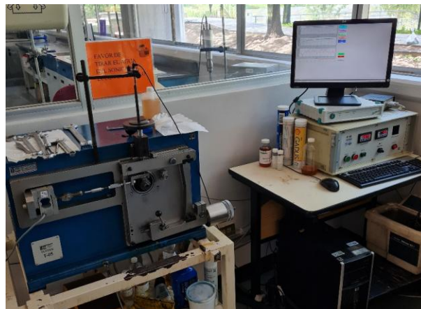
Fig. 1. T05 Block-on-Ring Wear Tester machine used for the testing.
