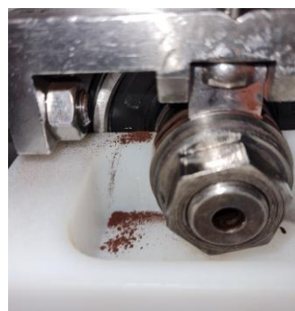
Fig. 11. Debris after testing samples from combination B.
