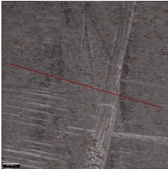
Fig. 17. Surface zone of combination A used to evaluate profile and roughness.
