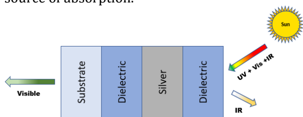
Fig. 13 Thin film multilayer Dielectric / Metal / Dielectric [21] (Adapted with permission from Publisher)
