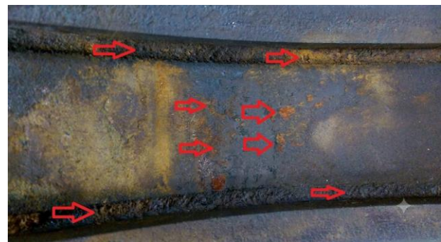
Fig. 5. Raceway region showing cavitation wear in the direction of maximum load.
