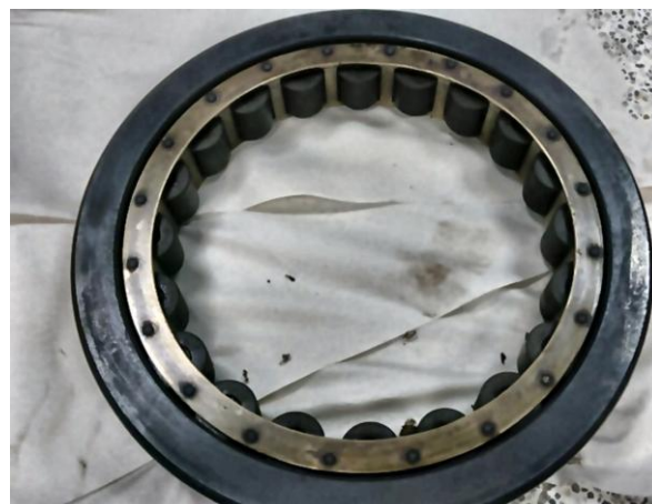
Fig. 1. NU240 bearing after cleaning following the ASTM procedure.
