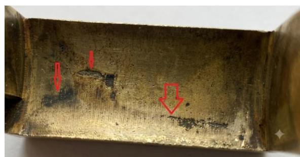
Fig. 10. Wear present on the bronze cage, resulting from contact between metal parts and deficient lubrication.
