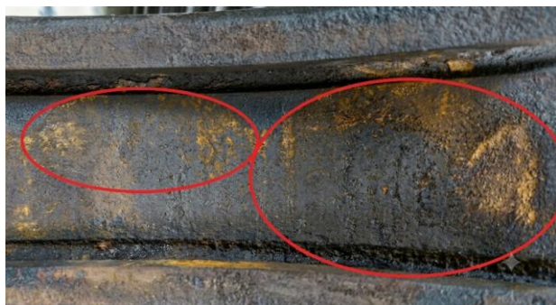
Fig. 7. Adhesive wear present on the steel raceway, resulting from direct contact between metal surfaces.
