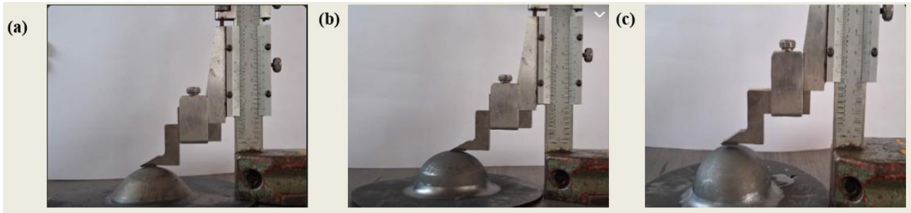
Fig. 5. Measurement of deep drawn cups using vernier height gauge (a) 250 °C, (b) 300 °C and (c) 350 °C.
