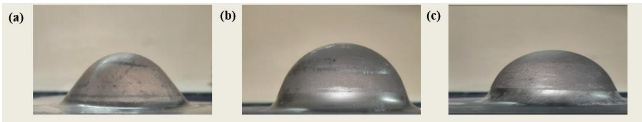
Fig. 4. Deep drawn cups drawn at the temperatures (a) 250 °C, (b) 300 °C and (c) 350 °C.
