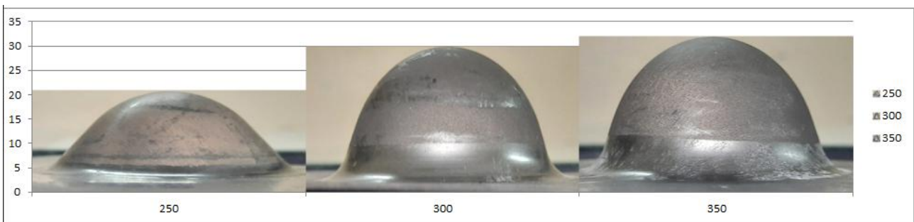
Fig. 6. Comparison of depth of deep drawn cups in mm drawn at 250 °C, 21 mm, 300 °C, 30 mm and 350 °C, 32 mm.
